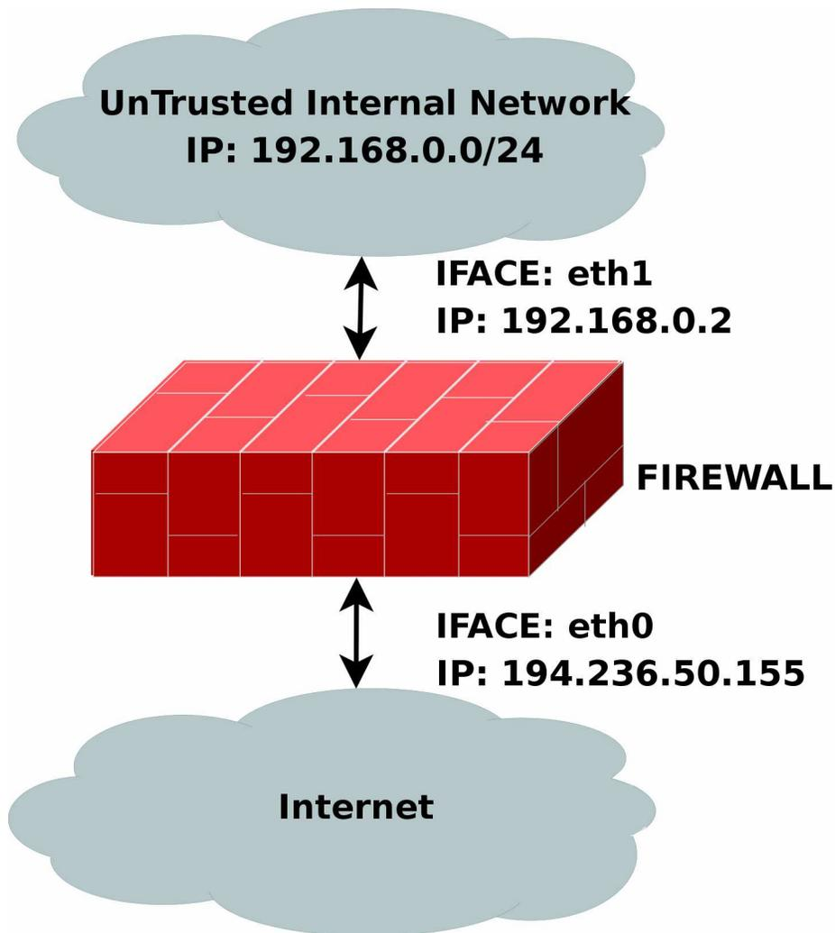
The rc.UTIN.firewall.txt (<http://iptables-tutorial.frozentux.net/scripts/rc.UTIN.firewall.txt>) script will in contrast to the other scripts block the LAN that is sitting behind
