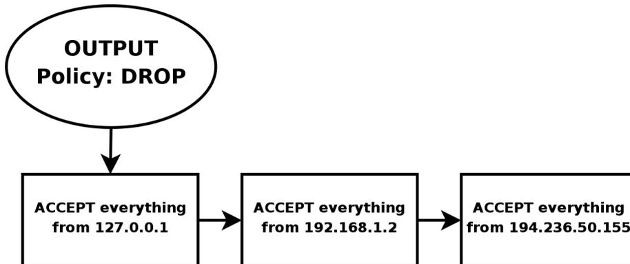
Finally, we have the firewalls *OUTPUT* chain. Since we actually trust the firewall quite a lot, we allow pretty much all traffic leaving the firewall. We do not do any specific user blocking, nor do we do any blocking of specific protocols. However, we do not want people to use this box to spoof packets leaving the firewall itself, and hence we only want to allow traffic from the IP addresses assigned to the firewall itself.
