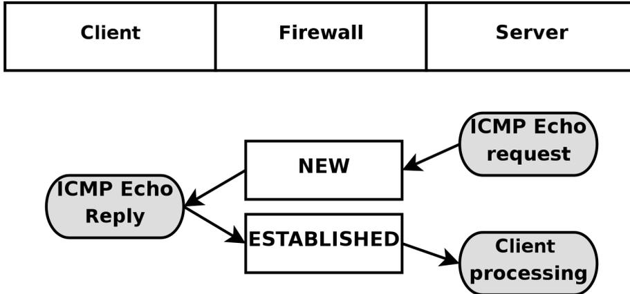
As you can see in the above picture, the host sends an *echo request* to the target, which is considered as **NEW** by the firewall. The target then responds with a *echo reply* which the firewall considers as state **ESTABLISHED**. When the first echo request has been seen, the following state entry goes into the `ip_contrack`.
