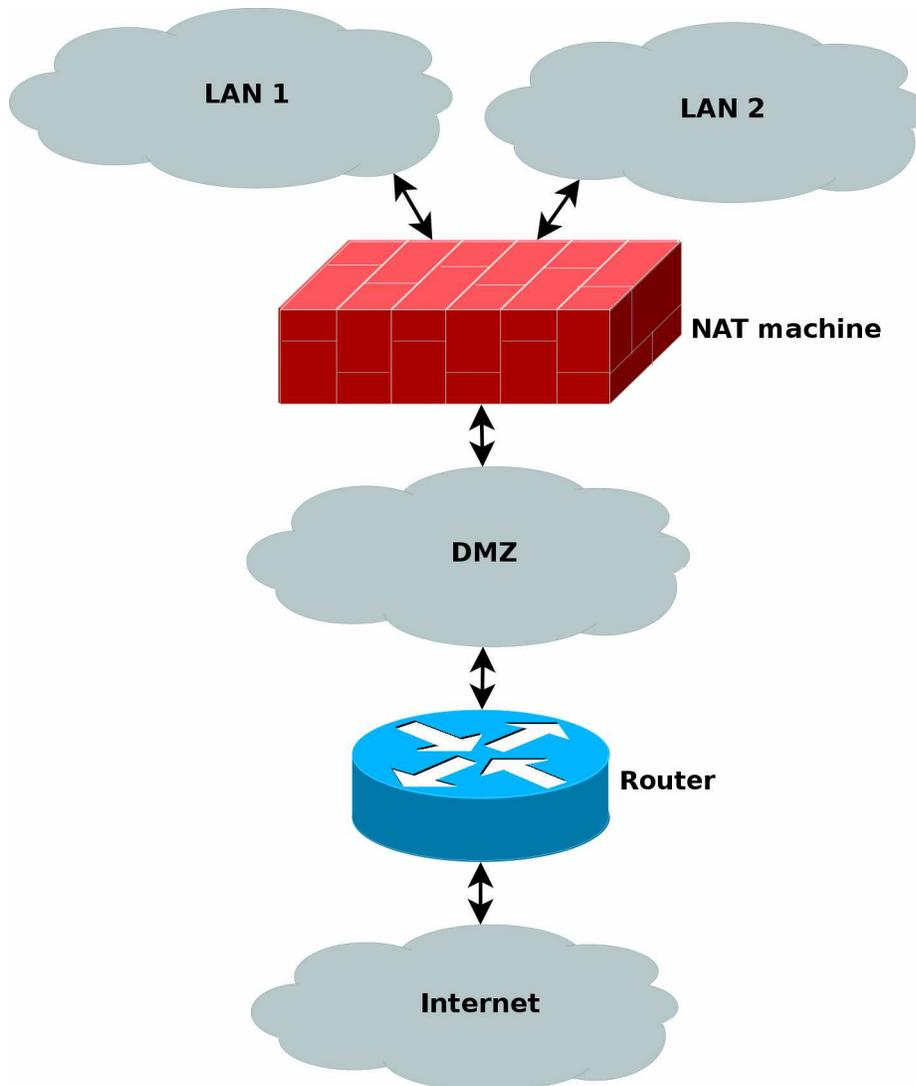
All the normal traffic from the NAT'ed networks will be sent through the DMZ directly to the router, which will send the traffic on out to the internet. Except, yes, you guessed it, webtraffic which is instead marked inside the netfilter part of the NAT machine, and then routed based on the mark and to the proxy machine. Let's take a look at what I am
