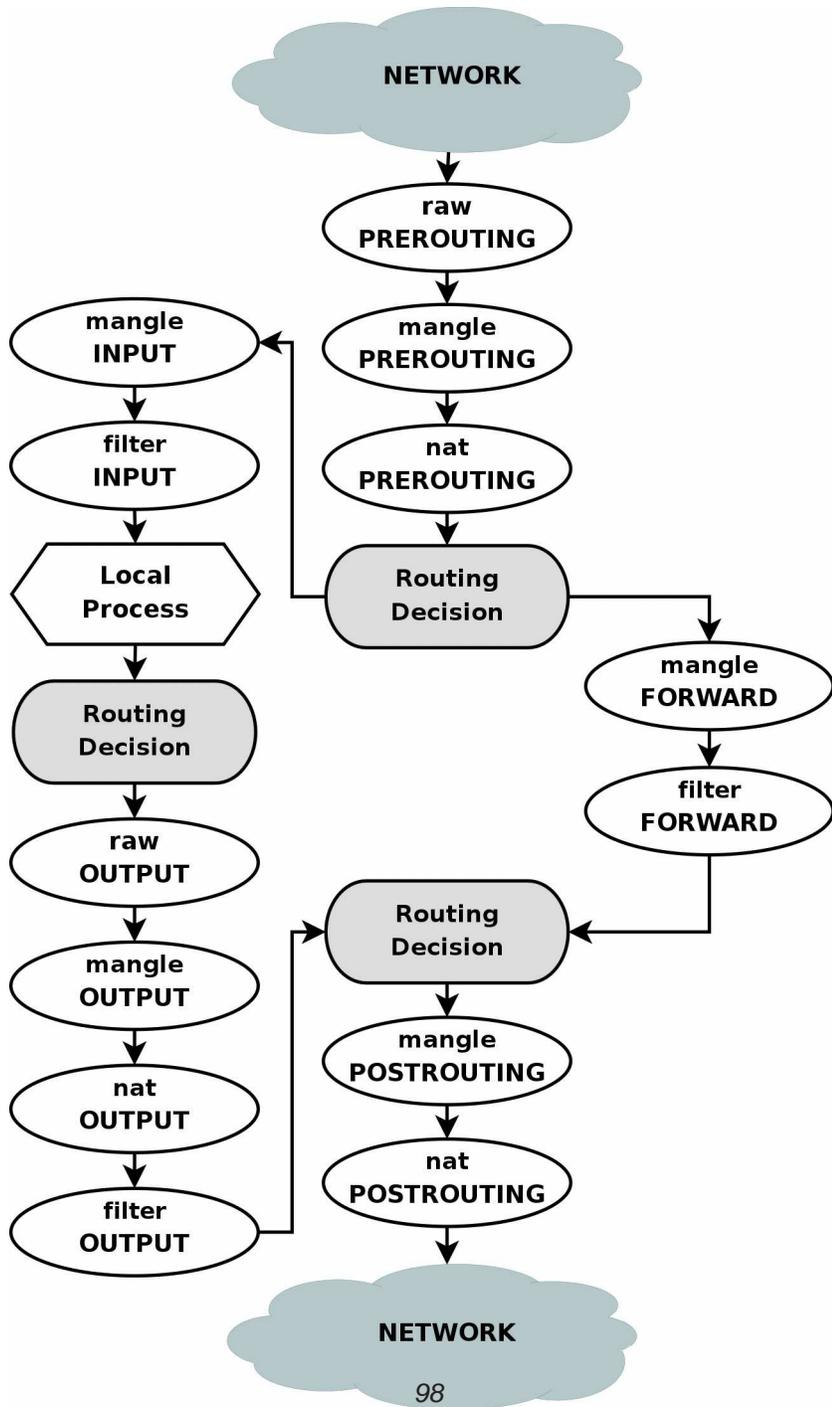
To clarify this image, consider this. If we get a packet into the first routing decision that is not destined for the local machine itself, it will be routed through the *FORWARD* chain. If the packet is, on the other hand, destined for an *IP address* that the local machine is listening to, we would send the packet through the *INPUT* chain and to the local machine.
