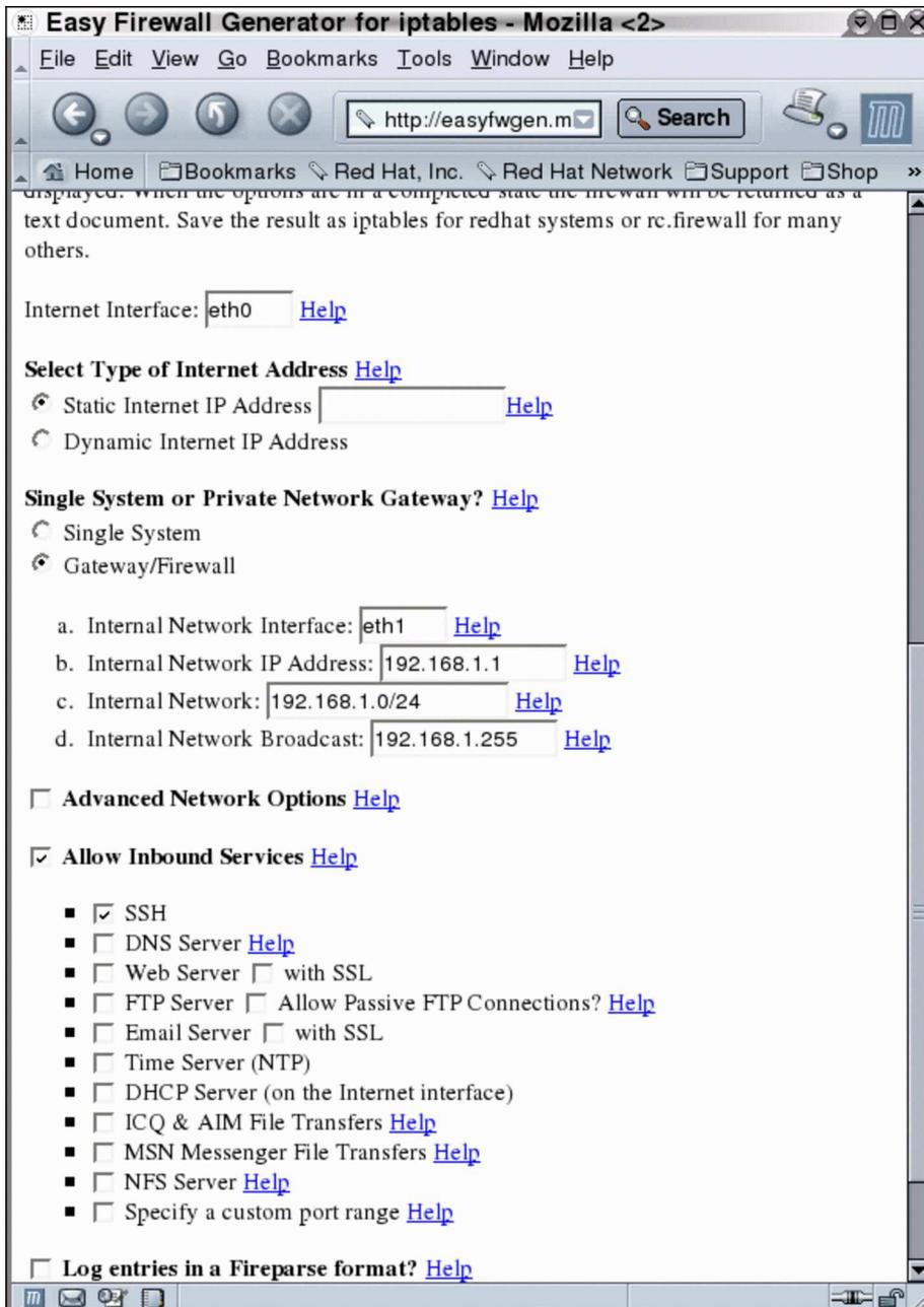
This screenshot shows one of the final stages of configuring the firewall script that is about to be created by the script. You can find more information, and a working version of the Easy Firewall Generator at <http://easyfwgen.morizot.net/>.
